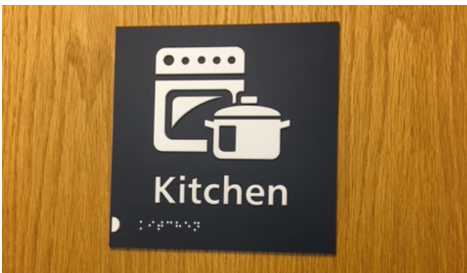
Image 16 – In addition to contrasting text and braille, relevant embossed images can also be used to provide information.
