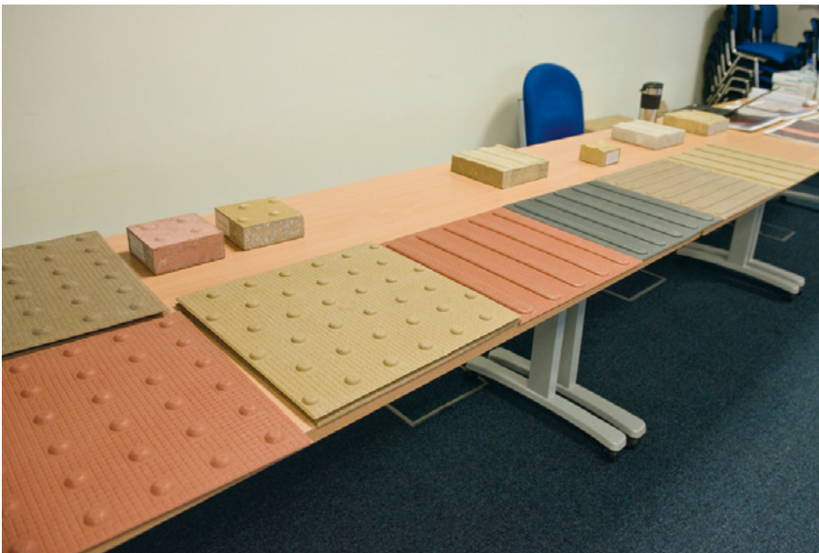
Image 3 - Tactile paving comes in different types and materials. This image shows blister, guidance and corduroy vinyl paving in light and dark colours.
