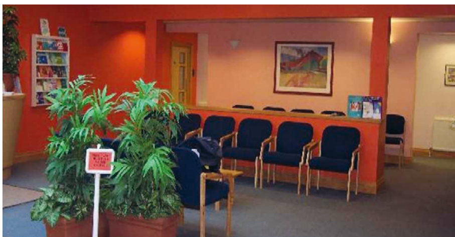
Image 17 – Using different textured flooring in contrasting colours can help people with sight loss identify different areas within a building. In this image, the walkway is tiled and the waiting area carpeted.
