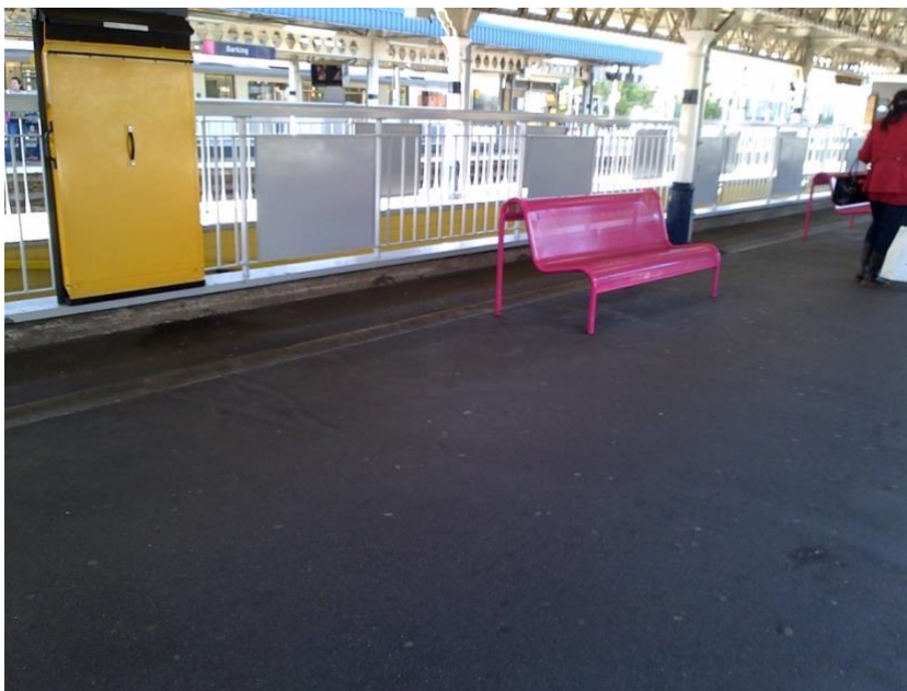
Image 23 - Train station platforms should have minimal furniture and clutter. Seating should contrast against its surroundings, so it is easy to locate.
