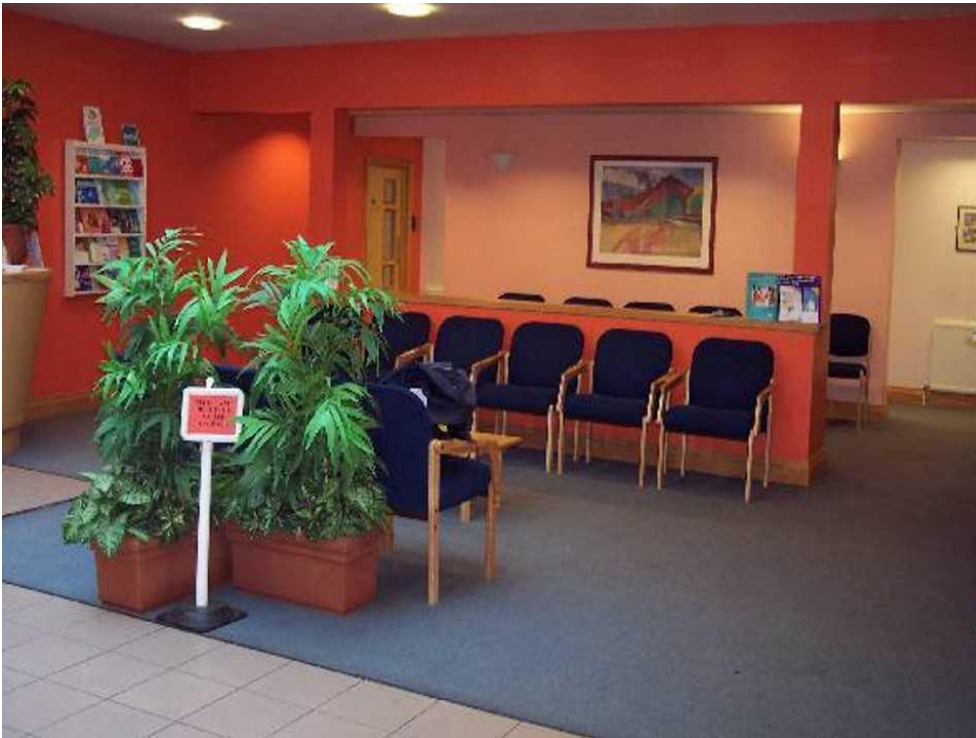
Image 17 – Using different textured flooring in contrasting colours can help people with sight loss identify different areas within a building. In this image, the walkway is tiled and the waiting area carpeted.
