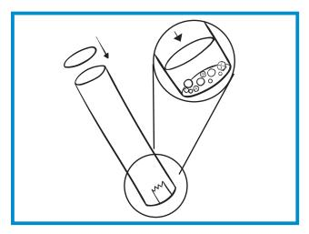
**4.** Put the frosted plastic disc on top of the beads etc.
