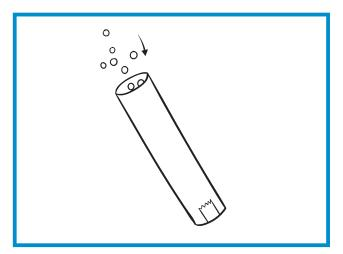
3. Pour your beads etc into the tube so they sit on top of the transparent plastic disc. Allow them to have enough room to move about.
